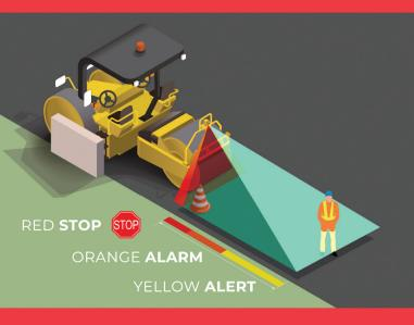
A first for the asphalt roller industry, Guardman® detects personnel, equipment, or objects behind the roller. The operator is warned progressively and if no action is taken automatically brakes when a collision is imminent.
