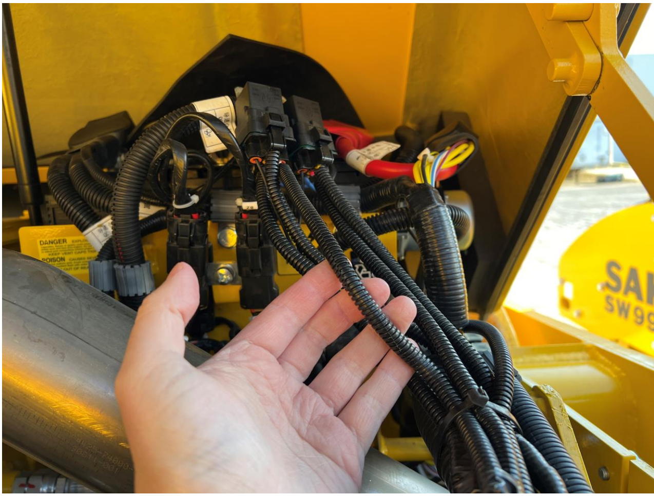
Runs back from relay to deck and up to the button switch
