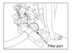
(**Fuel tank** (YANMAR and KUBOTA engine mounted models only)
