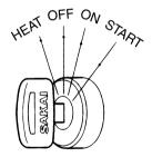
START: The engine is cranked and gets started. The moment the engine has started, release the key. It will automatically return to the "ON" position.
