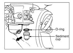
(4) **Fuel filter** (KUBOTA engine mounted model only)
