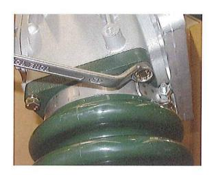
(2) Pull off the pin that connects con rod and the piston, and remove the crank case assembly.
