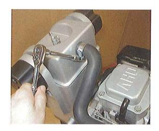
(2) Taking off the mounting bolts (10 pcs.) at the bottom and remove the engine guard.
