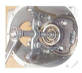
(6) Remove the snap ring that is fixed on the pinion gear.
