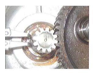
(7) Remove the pinion gear with a hammer.
