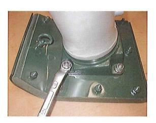
(3) Remove the bolts from shoe clamp. (top and bottom)
