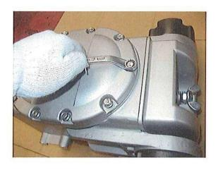
(4) Remove the snap ring from the con rod.
