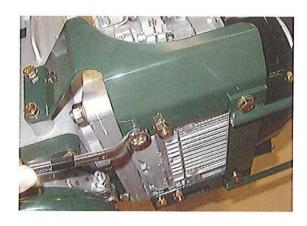
(3) Remove the nuts (4 pcs.) and dismount the engine.
