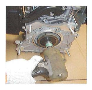
(2) Pull out the clutch using JIG.
