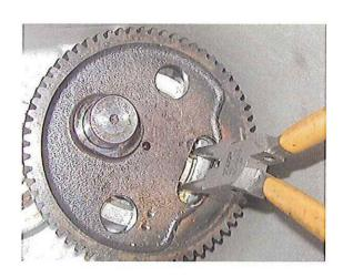
(9) Pull off the crank gear using jig.
