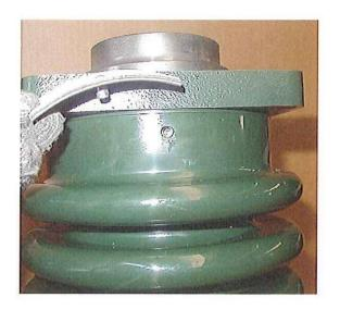
(5) Hit the bellows at the area as shown on the picture. Remove the outer cylinder and the bellows.
