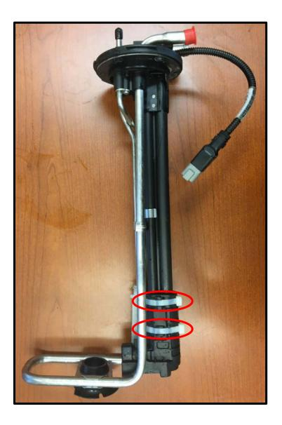
Using wire cutters. Cut both wire ties on the rubber boot.
