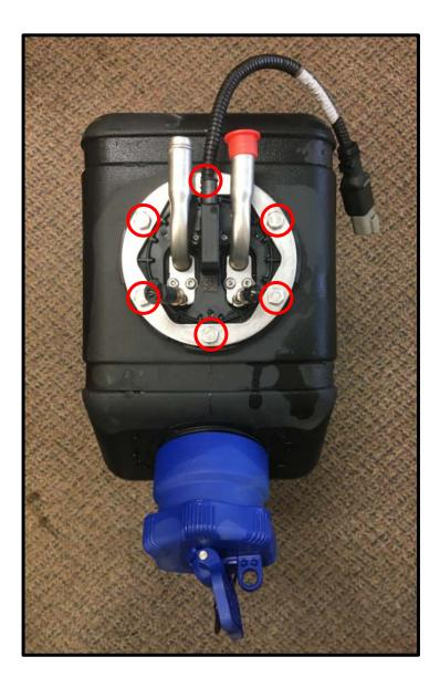
Use an 11mm wrench to remove all 6 bolts from DEF Header mounting plate.
