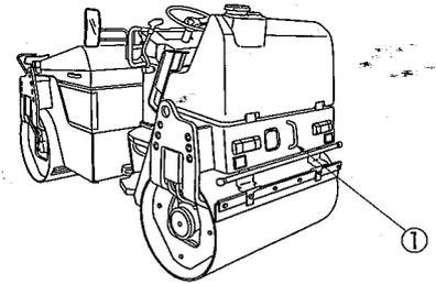
4) Place the unloader valve to the UNLOAD position (See "Unloader valve" on page 26). The unloader valve is located inside the engine room.
