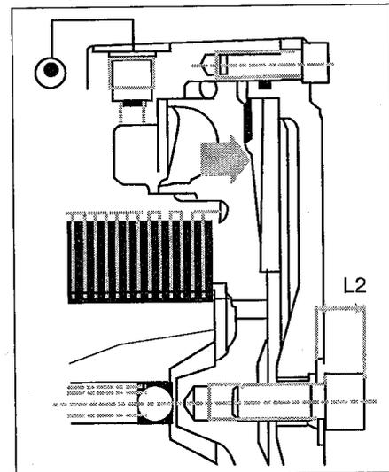
★ When the brake stroke exceeds the replacement standard shown below, replace all the friction plates and separation plates.
