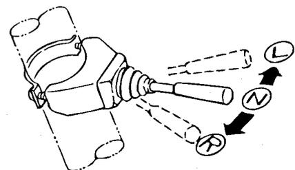
**NOTE:** The lever does not return to the OFF position even if the steering wheel is turned back.
