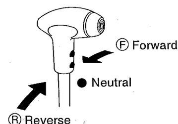
**NOTE:** The engine does not start due to an interlocking system if the F-R lever is not in the neutral position (●). Ensure that the F-R lever is in the neutral position (●) before starting.
