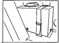
2) Turn the liquid spray quantity control valve on the liquid pipe clockwise to the utmost extent.
