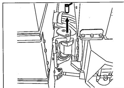
**NOTE:** Mount the removed lock pin in the innermost section of the step at the left of the vehicle.
