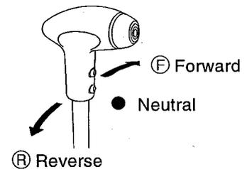
**NOTE:** The travel speed can be controlled by the throttle lever and F-R lever.
