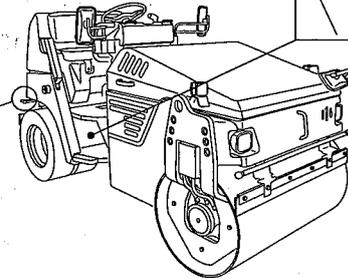
3) The liquid is sprayed over the tires. Press the liquid spray switch to spray, and the indication lamp of monitor display lights up. Spraying is shut off, and the indication lamp of monitor display is turned off when the switch is released. A valve is located on the liquid spray pipe to adjust spraying. To increase spraying, turn the knob clockwise. For reduced spray, rotate it counterclockwise.
