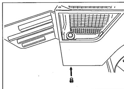
**NOTE:** When removing the water and sediment from the tank filled with the fuel, the fuel will gush out if the drain plug is screwed out completely.
