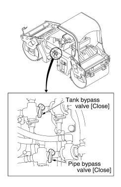
• If the valve near the filter is switched as shown at the right and one switch of either pump 1 or 2 is pressed, it becomes possible to spray to the front and rear drums with one pump (ECO mode / Back up mode).
