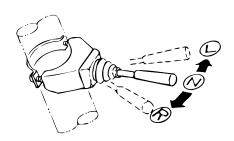
**NOTE**: The lever does not return to the OFF position even if the steering wheel is turned back.
