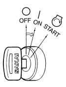
3) Start the engine after the engine warning lamp and the engine stop lamp have flashed once, then turned off.
