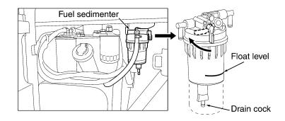
**NOTE**: After purchasing a new machine, drain water 50 hours after the initial operation.
