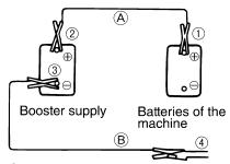
Connect to the engine block earth of the machine
