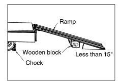
Decide the correct direction of run and conduct loading or unloading at low speed.
