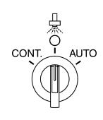
The indicator lamp  $\, \frac{1}{4} \,$  on the monitor display will turn on only while water is being sprinkled.
