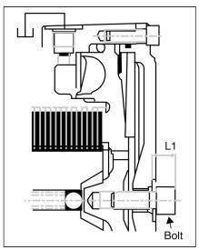
3) Inspection of brake stroke
