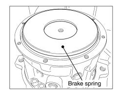
3) Preparation for removing brake piston
