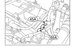
Be sure to replace the fusible link with one of the same capacity.
