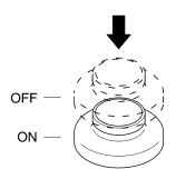
**NOTE:** If the liquid is not sprayed from the nozzle even when pressing the liquid spray switch, fully open the liquid spray quantity control valve (A) and press the liquid spray switch again to remove air in the circuit.
