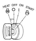
4) Turning the key to the START position makes the engine start. Release the key the moment the engine has started. The key will automatically return to the ON position.
