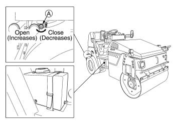
3) The liquid is sprayed over the tires. Press the liquid spray switch to spray, and the indicator lamp 🚊 on the monitor display lights up. Spraying is shuts off, and the indicator lamp 💂 on the monitor display is turned off when the switch is released. A valve is located the liquid spray pipe to adjust spraying. To increase spraying, turn the knob clockwise. For reduced spray, rotate it counter-clockwise.
