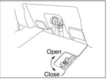
2) The water sprinkler switch can be used to switch between continual sprinkling and sprinkling in coordination with the F-N-R lever.
