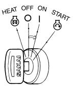
NOTE: The various warning lamps will turn on when the starter switch is turned to the ON position, and only the hydraulic oil filter warning lamp will turn off after that.
