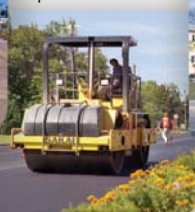
Vibratory Asphalt Rollers
