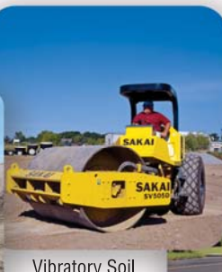
Vibratory Soil Compactors
